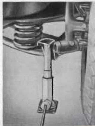
Jack pads front and rear make it easy for the owner himself to change a flat tire.
