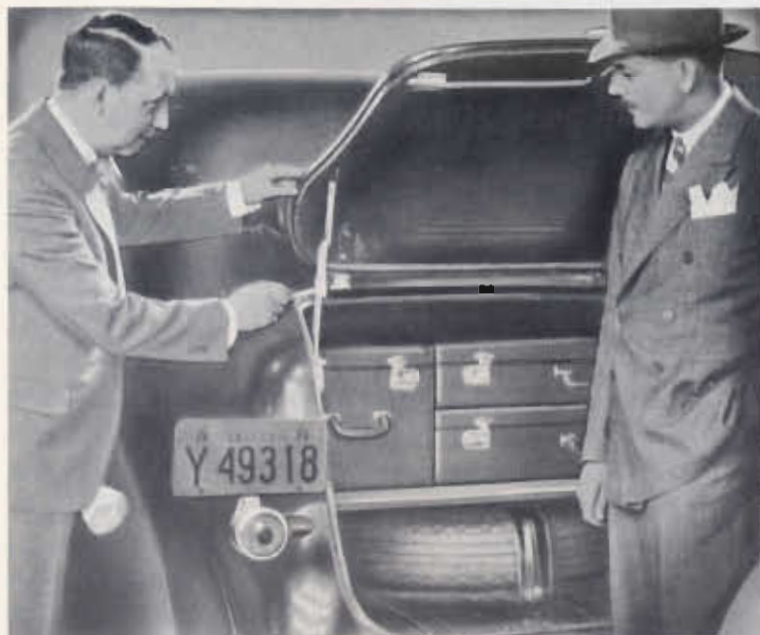
Raising the one-piece trunk lid locks this safety hinge. Another lift and it is automatically released.
