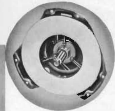
That hard-to-reach clutch release bearing has lubrication sealed in for its life.
