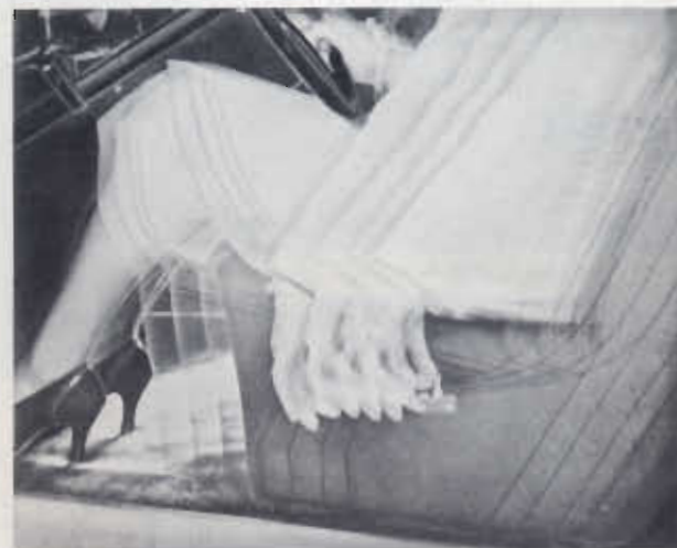
As the adjustable front seat is moved forward, the front edge of the seat cushion rises and the seat back tilts forward. A more comfortable position for the shorter driver is thus assured.
